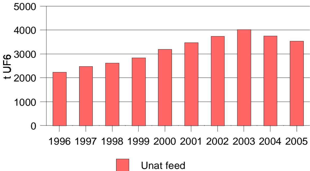
Fig. 2: Urenco Gronau UF6 feed input (after [Urenco 2006])
